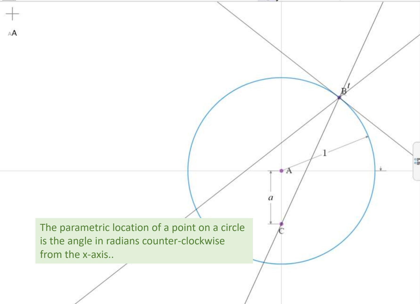
The parametric location of a point on a circle is the angle in radians counter-clockwise from the x-axis..
