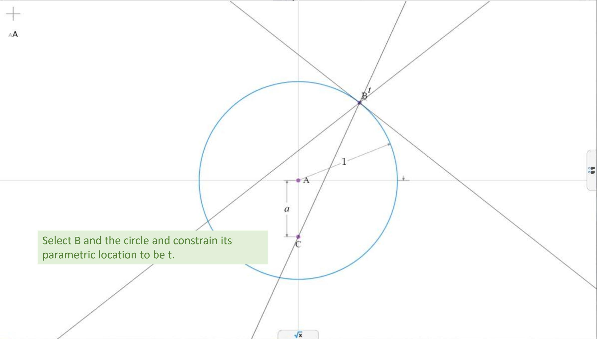
Select B and the circle and constrain its parametric location to be t.
