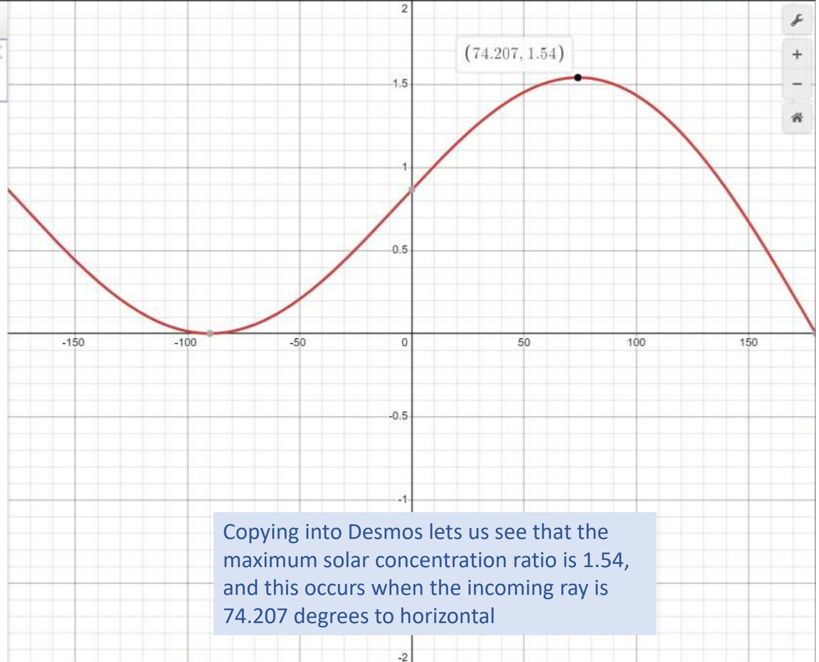
Copying into Desmos lets us see that the maximum solar concentration ratio is 1.54, and this occurs when the incoming ray is 74.207 degrees to horizontal
