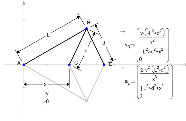
**Fig. 4** Input kinematics element specifies velocity and acceleration for the length constraint  $x$ . Output kinematic element measures cartesian velocity and acceleration of point D.
