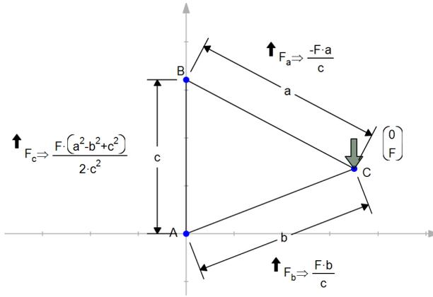
**Fig. 1** A triangular truss with force applied at B. Constraint forces are displayed for the three length constraints.
