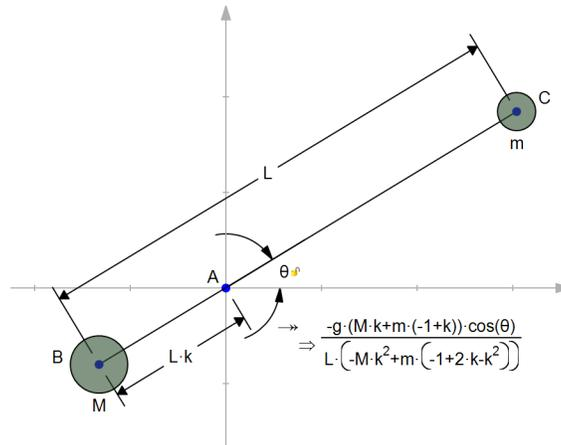
**Fig. 10** Acceleration in the angle  $\theta$  is displayed
