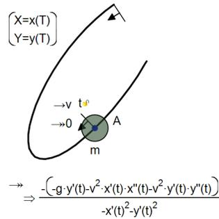
**Fig. 12** A mass is located at A which is constrained to be at parametric location  $t$  on the curve  $(x(t), g(t))$ . It is given parametric velocity  $v$ . The resulting parametric acceleration is displayed.
