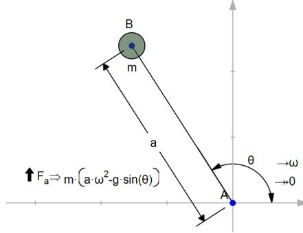
**Fig. 3** AB rotates in a vertical plane with angular velocity  $\omega$ . Reaction force in the length constraint is shown. One term is due to gravity acting on the mass, the other term is a centripetal pseudoforce introduced by the accelerating mass.
